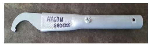
Another hint is if you value your hands and to make adjusting heaps easier is to extend the Hagon Spring Adjusting Spanner, and apply some silicon spray to the Adjusting thread and spray some between the Castellations on the adjusting nut to get at the top surface of the spring and make it easier to adjust.
